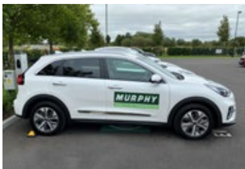
Our fleet of Kia e-Niro EVs emit zero emissions and can achieve 282 miles on a single charge from a 64 kWh battery pack. A 50kW public charger will take an e-Niro EV from 0-80% in just 1 hour 15 minutes, or a 100kW charger will do it in just 54 minutes.
